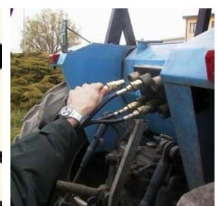
Elettroil connection to quick-fit couplings of the tractor
